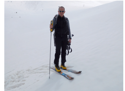
Fig. 2: view of penetration testing with automatic Avatech SP2 probe
